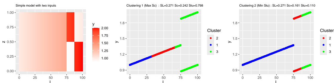
Figure 1: Clustering result of a simple model for the two criteria. Left: model definition; Middle: clustering based on S_c ; Right: clustering based on S_u^T .
